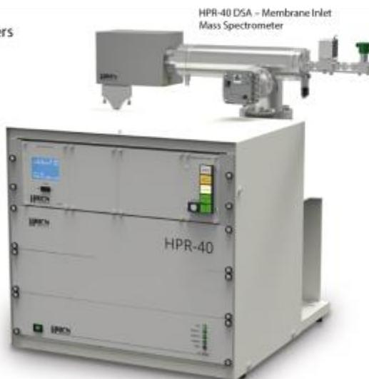
HPR-40 DSA - Membrane Inlet Mass Spectrometer
